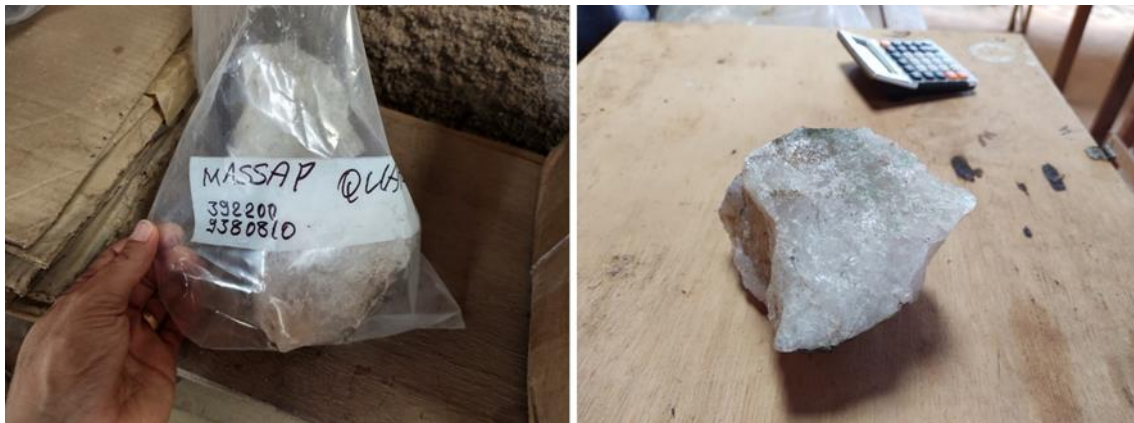
Figure 11-11: Coarse Blank Material to be Applied as Quality Control sample for ValOre's Pedra Branca Project (Source: Fábio Valério Câmara Xavier, Geologist, MAIG – this report).
