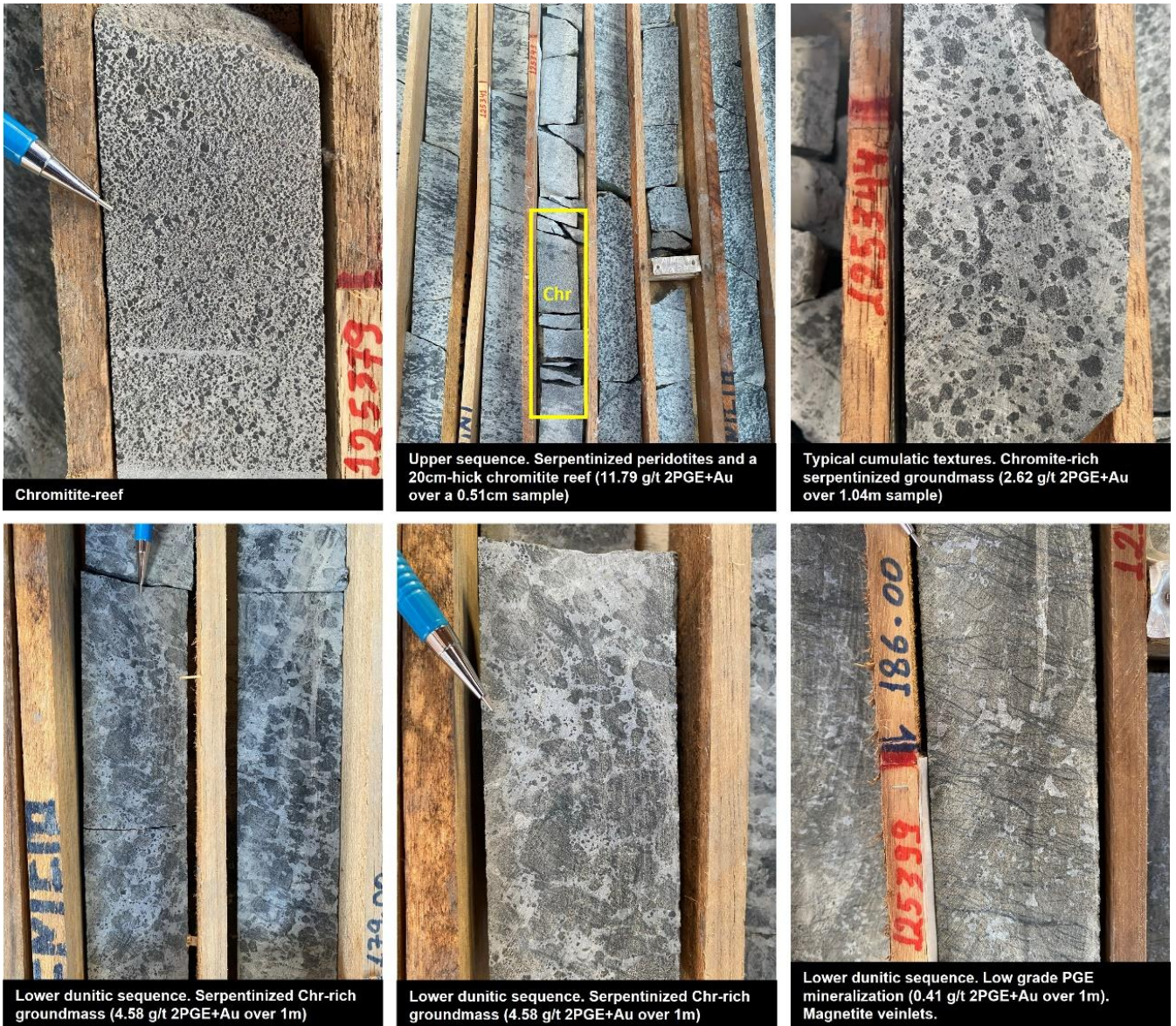
Figure 1-5: Typical Cumulate Textures in Mineralized Metaperidotites and Metadunites from the Trapiá Deposit. (Source: Thiago Diniz, P.Geo – ValOre).
